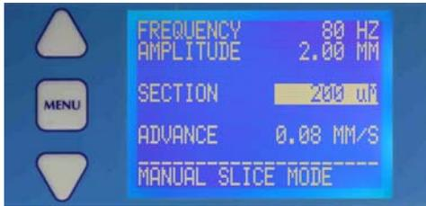
The 'RETURN' key may now be used to retract the head to the position you had selected as the start position above. Before the head retracts the bath will be lowered so that the blade does not drag across the surface of the specimen. After the head has been retracted the bath will be raised to its previous position and then raised once more by the thickness of the section in readiness for another cut.
