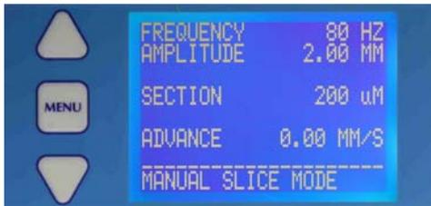
Press the 'MENU' key to go to the display shown. This is the normal operating display.
