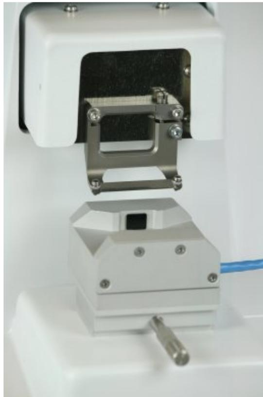
When the calibration device is plugged into the instrument its presence will automatically be detected and it will take control of the amplitude and frequency settings, adjusting them to a magnitude that allows best adjustment of the blade alignment error. The alignment process also automatically moves the blade so that the cutting edge is in its optimal position relative to the calibration device for best alignment evaluation.
