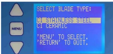
You must now choose which type of blade you want to calibrate. Scroll to the appropriate blade using the  $\Delta$  or  $\nabla$  keys and press 'MENU' to select.
