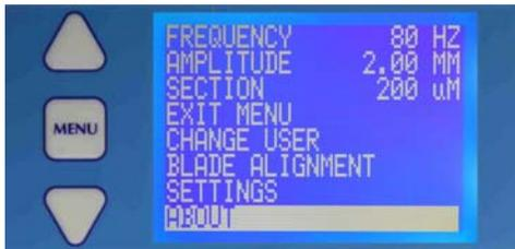
Use the  $\triangle$  or  $\nabla$  keys to scroll to the line 'ABOUT' and press the MENU key.
