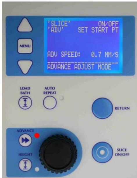
Press the 'ADVANCE' key and using the rotary knob to control the advance speed. Press the 'SLICE' key to switch the movement on or off.
