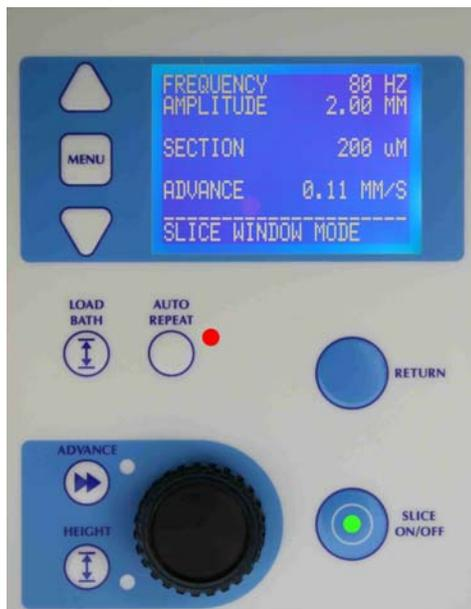
When a satisfactory cut window has been made, press the 'AUTO REPEAT' key once until the slice window screen is displayed. The led adjacent to that key will be illuminated in red as a warning.
