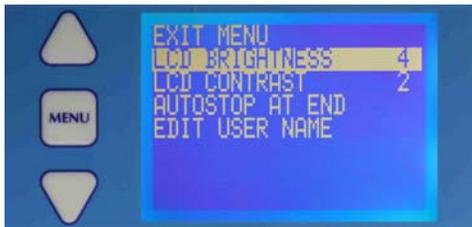
Use the  $\Delta$  or  $\nabla$  keys to scroll to line required and press the MENU key. The feature value will be highlighted and may be adjusted using the  $\Delta$  or  $\nabla$  keys. Press the MENU key to confirm the change.
