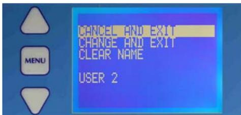
Use the  $\Delta$  or  $\nabla$  keys to scroll to the line (in the example shown) 'USER 2'. Pressing 'MENU' again will cause the 1<sup>st</sup> letter of the name to be highlighted. The rotary knob can now be used to scroll through the alphabet to select a new letter or symbol. Press the  $\Delta$  to confirm and move to the next letter position; use the rotary knob to select a new letter. ( $\nabla$  selects the previous position). Continue until the new user name is acceptable.
