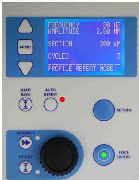
When a satisfactory cut profile has been made, press the 'AUTO REPEAT' key twice until the profile repeat screen is displayed. The led adjacent to that key will be illuminated in red as a warning.
