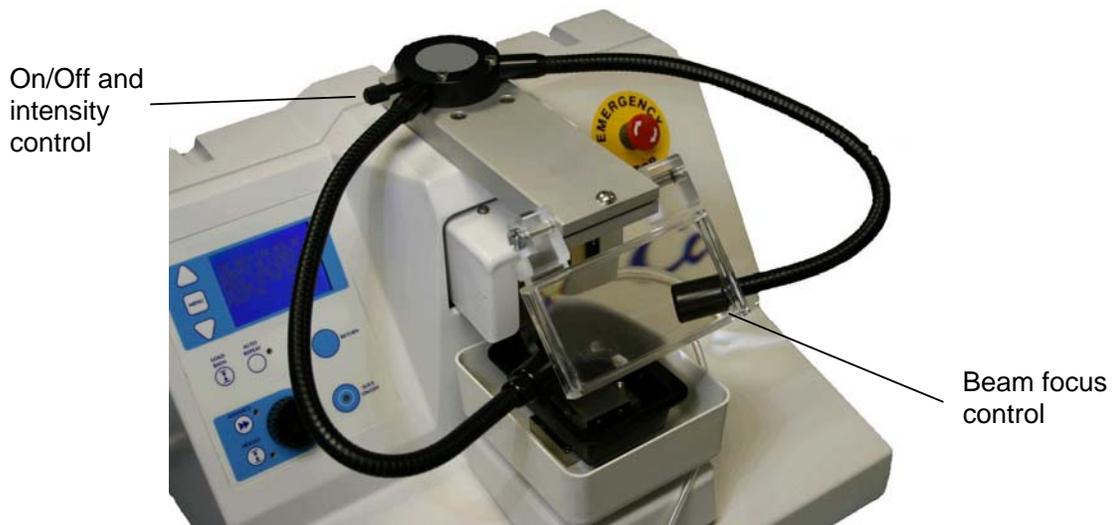
The light source can be switched on and the light intensity controlled via a combined rotary switch/potentiometer on the body of the light source where the flexible arms are mounted.
