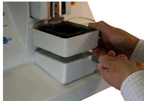
Pressing 'LOAD BATH' keypad will cause the table to rise to a preset (nominal) position.
