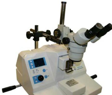
7000smz fitted with the stereoscopic microscope
