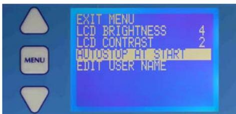
Use the  $\Delta$  or  $\nabla$  keys to scroll to the AUTOSTOP line. Press the MENU key to toggle between AUTOSTOP AT END or AUTOSTOP AT START. Use the  $\Delta$  or  $\nabla$  keys to scroll to line EXIT MENU and press the MENU key to get back to the basic menu display.
