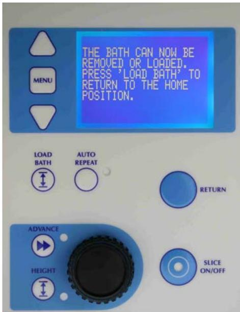
Once the table has reached its lowest position the display will be as shown. The specimen bath is located on the rising table by a convergent double dovetail slideway and clamping screw.
