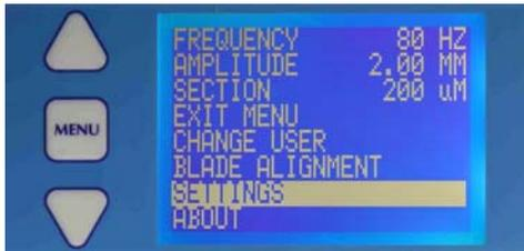
From the basic menu screen use the  $\Delta$  or  $\nabla$  keys to scroll to the line 'SETTINGS' and press the MENU key.
