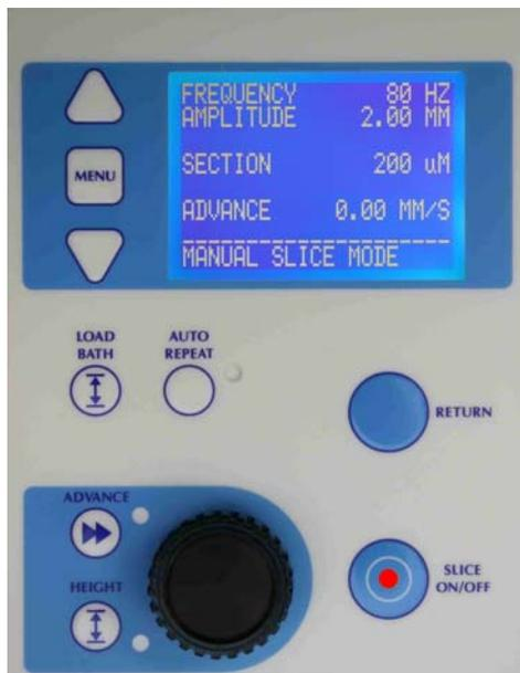
Press the 'SLICE ON/OFF' key to commence the cut. The 'SLICE ON/OFF' key will now change to a red illumination. Use the rotary knob to control the advance speed as the blade moves through the tissue.
