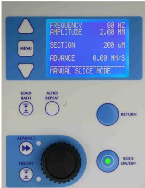
Note that the 'SLICE ON/OFF' key is now illuminated green and the advance speed as shown on the display is 0.00mm/s.
