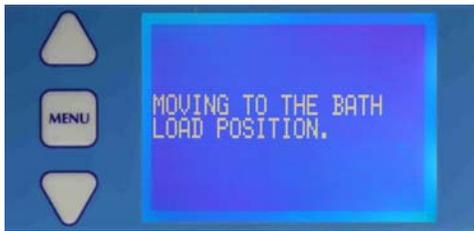
Press the 'LOAD BATH' key and the display will change to that shown. The bath table will be moved to its lowest position to allow a specimen bath to be loaded (or an existing one removed).
