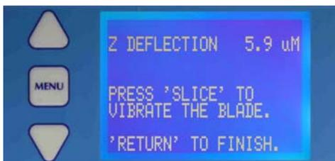
The display will now change to that shown on the left. Note that the uppermost line shows the current Z axis (vertical) deflection. At this point it indicates zero because the blade is not moving.
