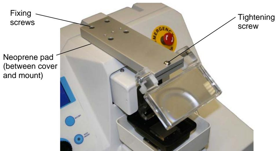
To adjust the lens, slacken the tightening screw and pivot the lens as required. Re-tighten the screw.
