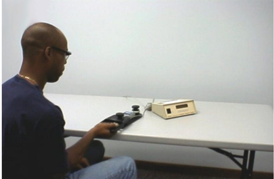
1. Attach the load cell to the grip test unit by removing the two large black screw-knobs, placing the load cell in position, and replacing and tightening the screw-knobs.
