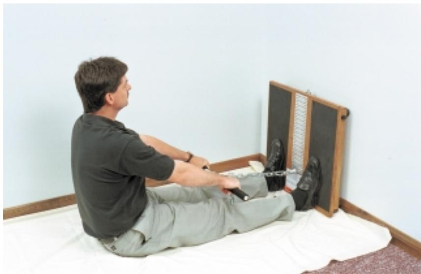
1. The lift bar is attached to a chain link that places the bar 17 inches from the base of the platform. The same chain setting is used for all subjects. The handle should be attached to the 8th link in the chain.
