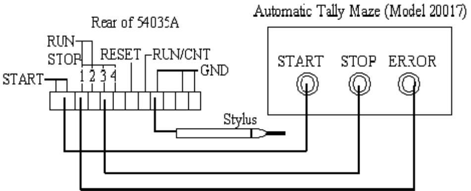
Figure 4: 54035A/20017 Connection diagram
