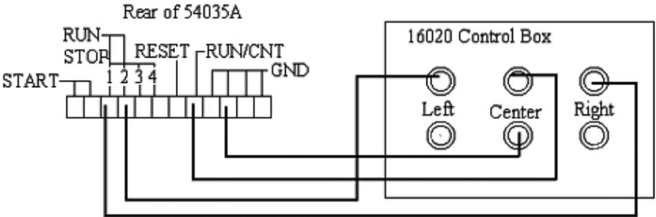
Figure 2: 54035A/16124 connection diagram
