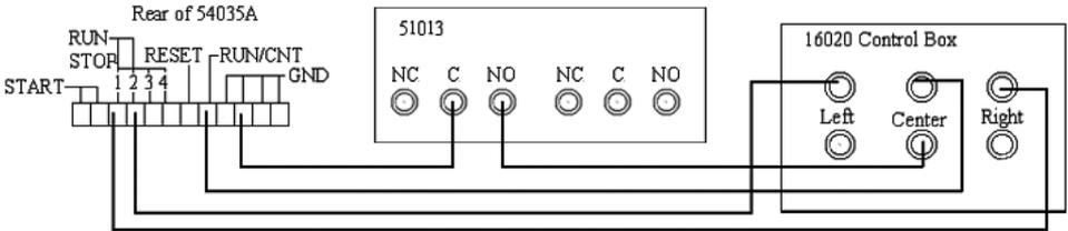
Figure 3: 54035A/16125 connection diagram
