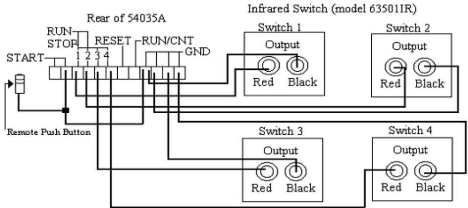
Figure 5: 63501IR/54035A Connection Diagram
