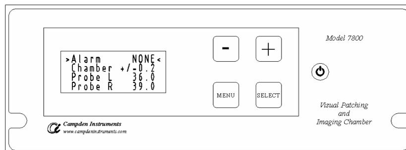
Figure 16: Controller front panel – Alarm screen
