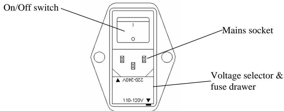
**Figure11: Mains inlet/voltage selector (example shown is set to 110-120V)**
