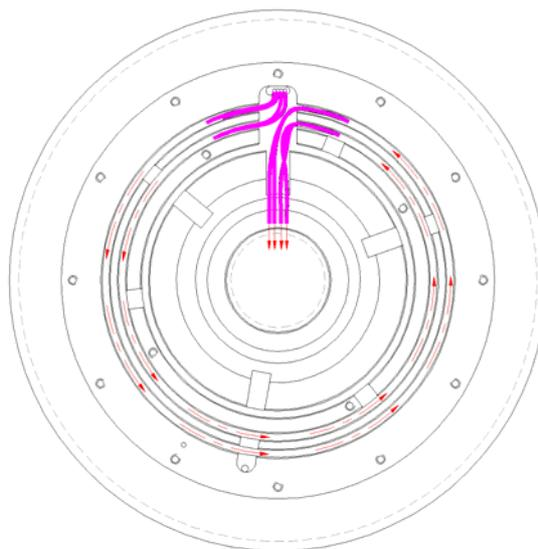
Figure 3: Routing of Perfusate Tubing
