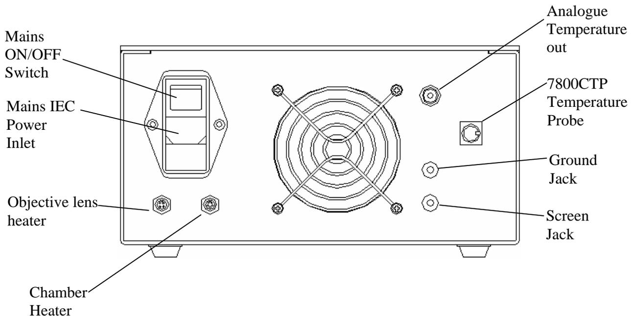
**Figure 12: Rear view of heater controller**
