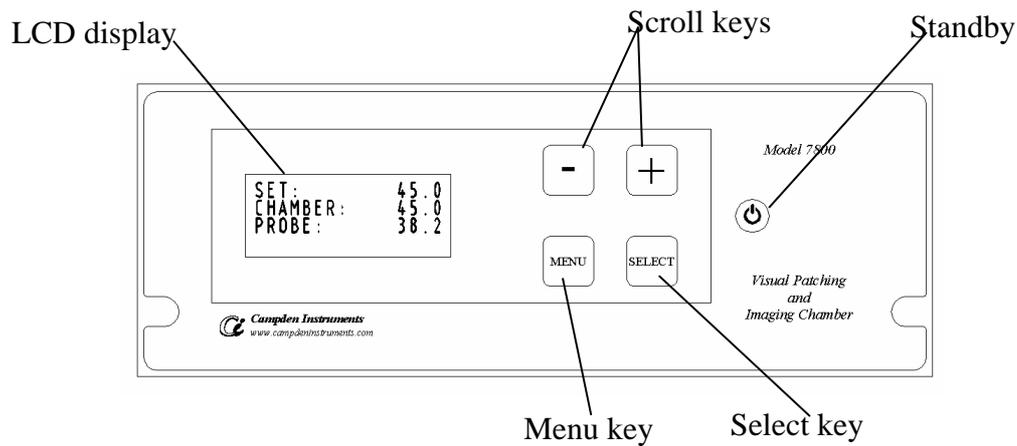
**Figure 13: Controller front panel (as used with a slice chamber)**
