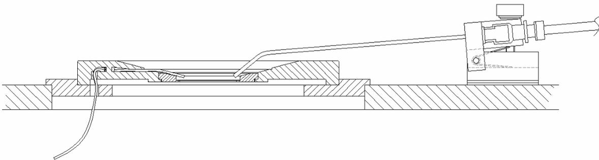
**Figure 10: Positioning the Suction Needle**
