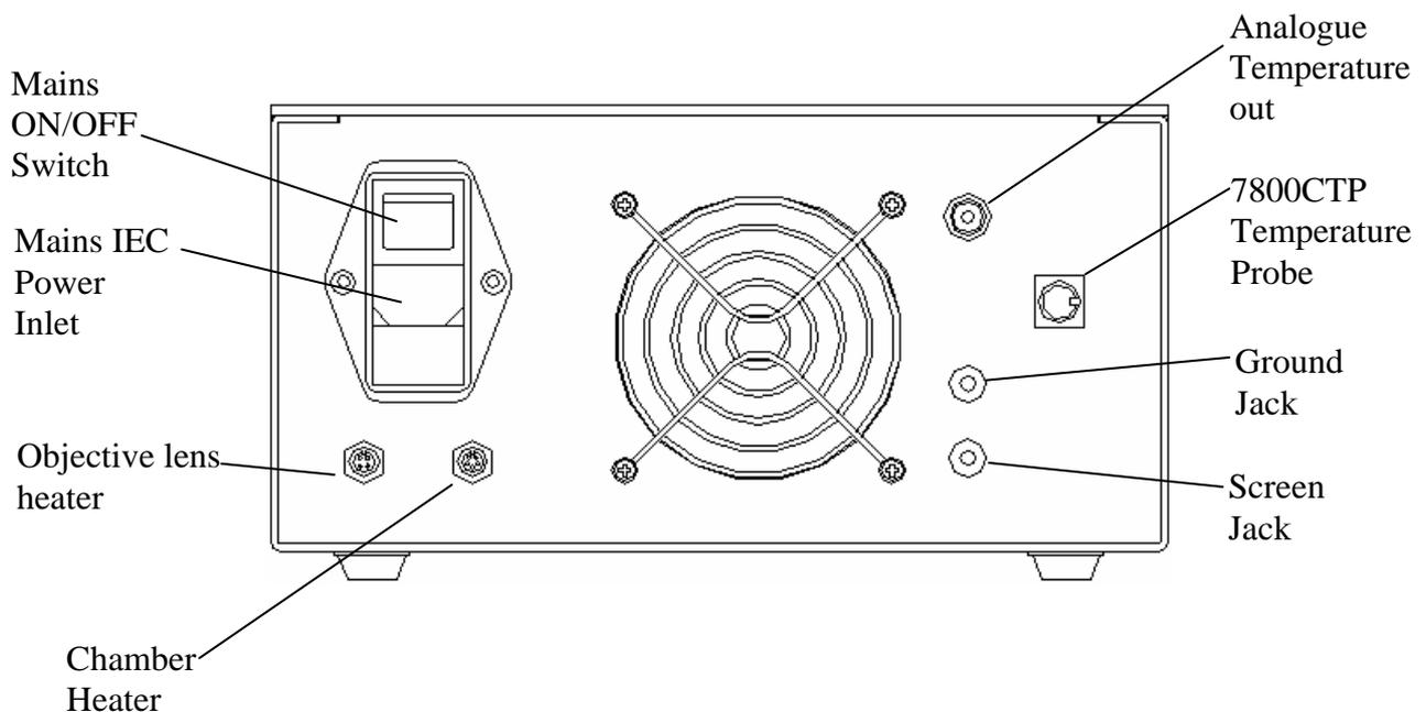
**Figure 12: Rear view of heater controller**
