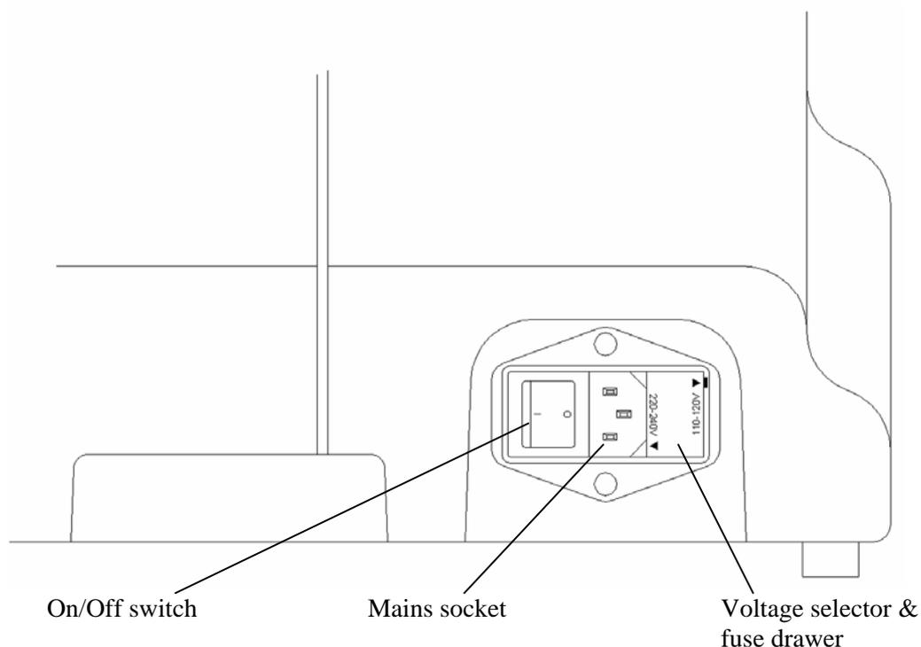
**Figure 3** Voltage supply selector (example shown is set to 110-120V)
