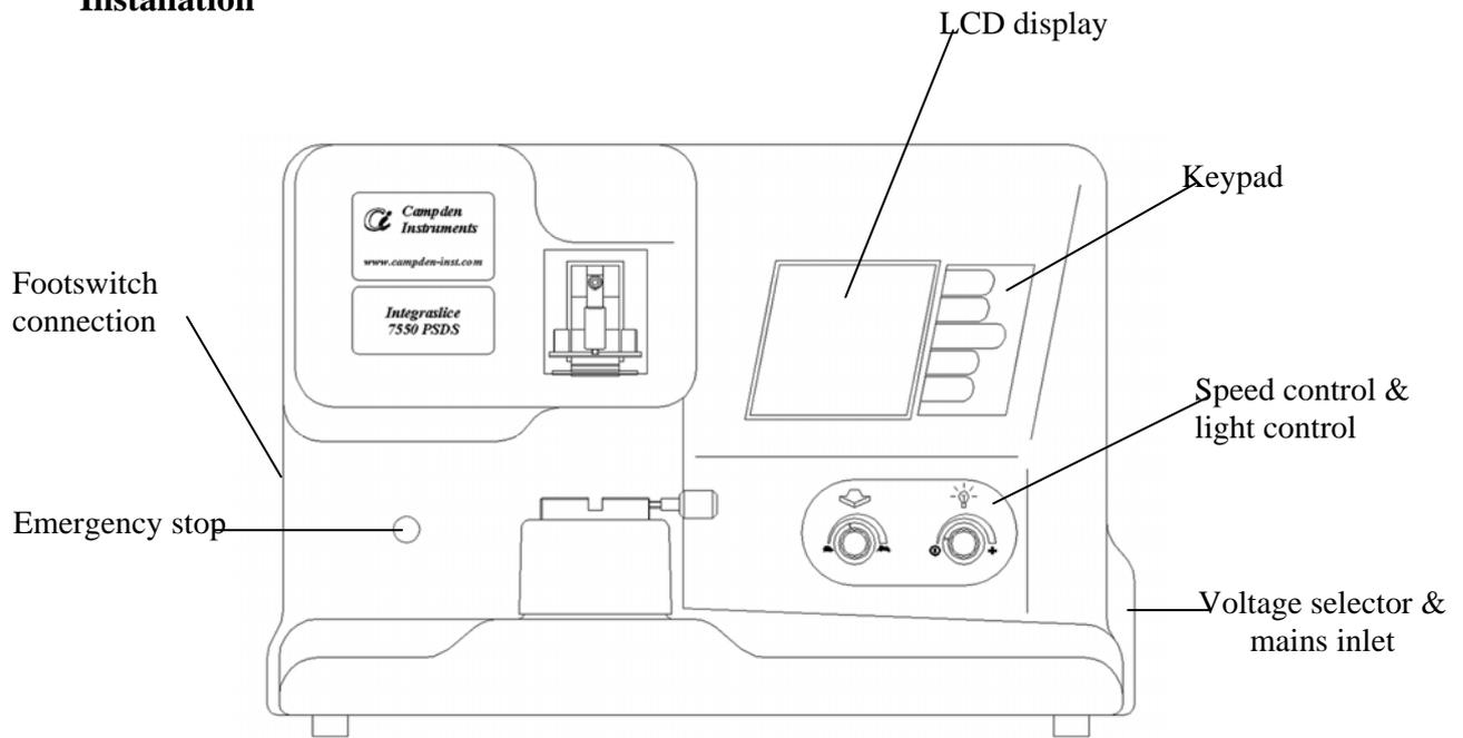
**Figure 1** Front view of the Integraslice
