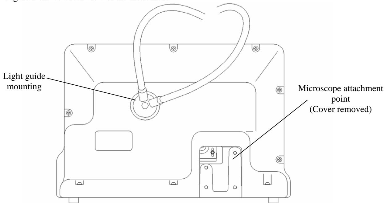
**Figure 2** Rear view of the Integraslice
