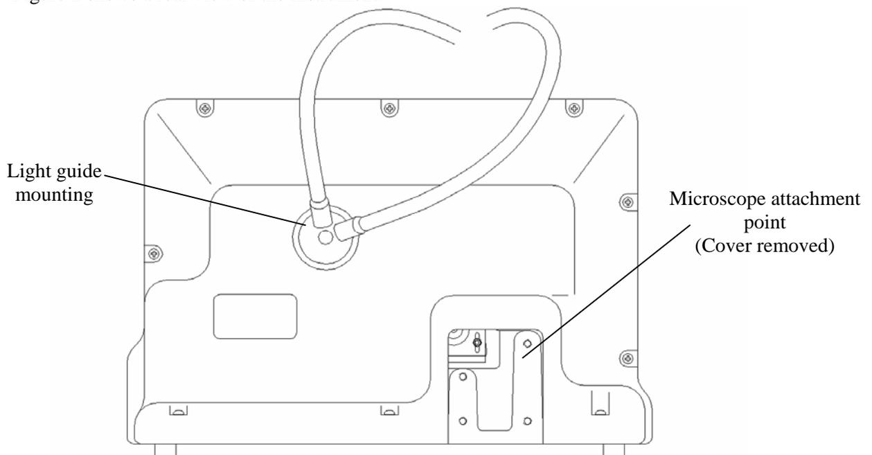
**Figure 2** Rear view of the Integraslice
