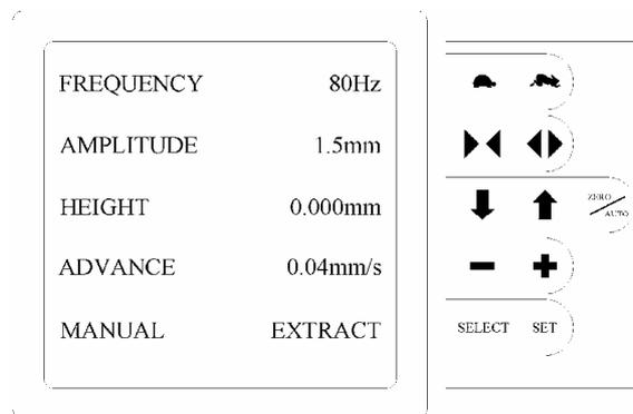
**Figure 8** Manual mode display
